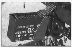
Kent Lomont's bracket permits use of the now more common .30-caliber ammo cans without the latching mechanism on the M1917A1 tripod.
